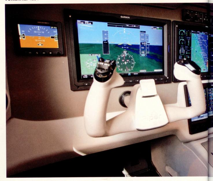
The Garmin G3000 dominates the Piper Altaire cabin and cockpit mock-up that is currently on tour (above). The G3000 features touch-screen data-entry pads (below the MFD). An L-3 Trilogy back-up display (left of the pilot's PFD) provides redundancy in the case of multiple screen or power failures. Engineers with roots from Hawker obsess over cockpit details, including (far right) light and ventilation positions, cockpit entertainment, and interior materials.
